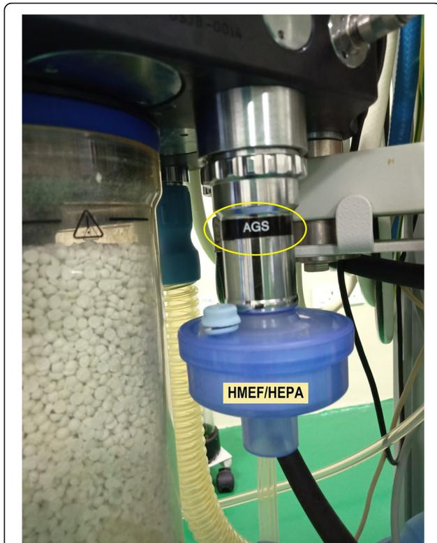
**Fig. 1** Dräger Fabius Plus anesthesia workstation—the heat moisture exchanger bacterial-viral filter (HMEF) is attached to the active gas scavenging (AGS) port (labeled on the machine by the manufacturer). HEPA, high-efficiency particulate air filter
